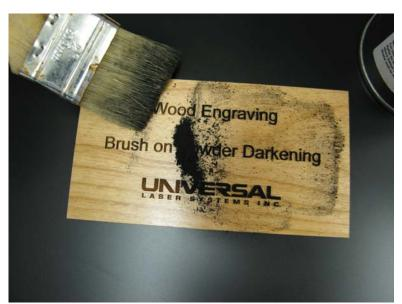
2. Brush into each groove then brush of excess powder and wipe surface clean.
