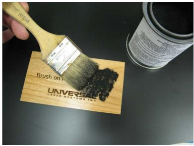
1. Remove engraving from laser system & brush in powder.
